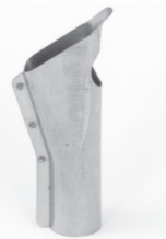
35271 Tack Welding Tip For tack welding two pieces together before adding filler rod. Use with 3/8" reducer.
