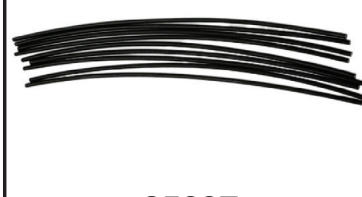
35697 Fiber-Flex Hot Melt Adhesive Rod (Pkg. of 9) Round, 3/16" Dia. x 12" Long, Black, "Universal" rod, works best with PP and TPO plastics.
