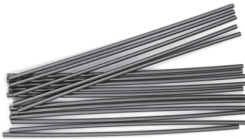
35297 ABS Welding Rod (Pkg. of 16) Round, 1/8" Dia. x 9" Long, Natural, for welding ABS plastics
