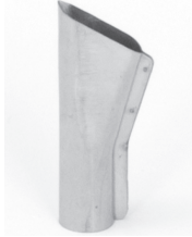
35296 3/4" (20 mm) Lap Welding Tip For lap welding plastic materials, such as PE, PVC, or Vinyl tarpaulin. Use with 3/8" reducer.
