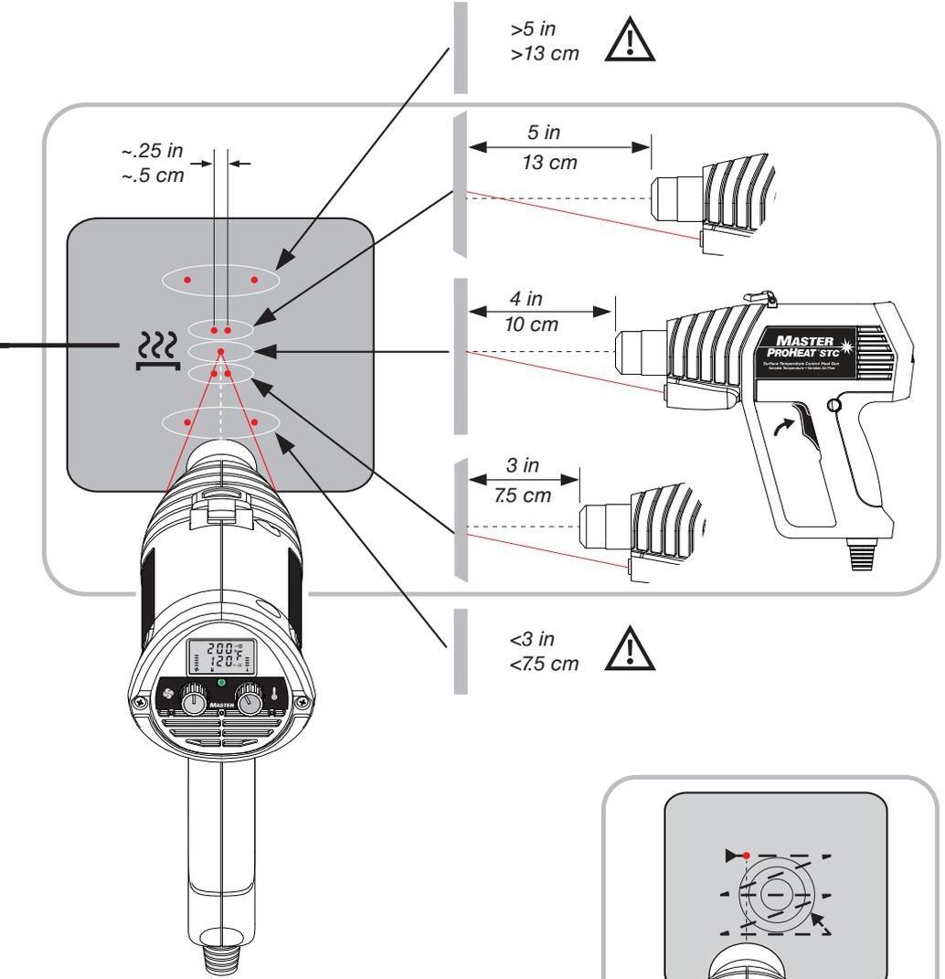
**NOTE:** Target surface temperature on the ProHeat STC can be dialed up to 500°F (260°C) in 10 degree increments. Thermal conductivity, emissivity and climate conditions may affect maximum heat range. Different material surfaces have varying capacities of absorbing heat. Users should independently evaluate the suitability of the product for their application.
